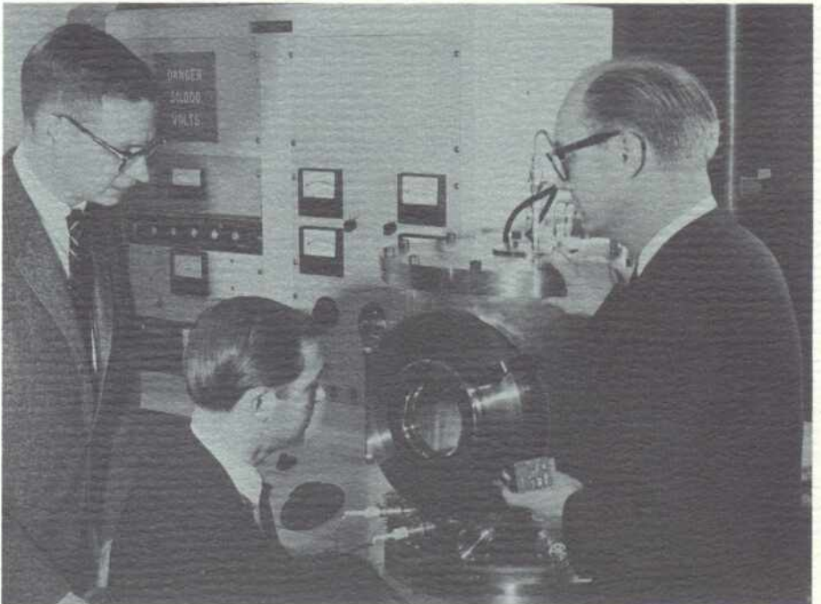
Techniques Lab management in front of high vacuum electron beam deposition system used in the fabrication of thin film devices. (Robert Baron, Director of Modular Products, left; Colin W. Knight, Manager of Techniques Lab, seated; T. Paul Bothwell, Vice President-Engineering, right).
