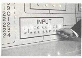
The computer demonstrator operates in parallel and uses a ten bit binary word. The bit positions are grouped from left to right in the following manner: The first bit is for sign — the next four bits indicate the particular OP code — the last five bits indicate the memory location.
