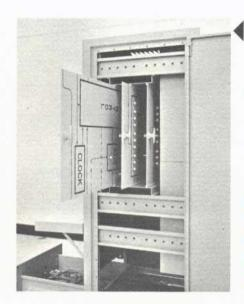
End view shows storage locations of the computer trainer panels. All panels, logic modules, patchcords and accessories are stored within the trainer when not in use.
