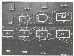
By simple patchcord wiring the instructor can synthesize a wide variety of logic operations, such as counter, shift register, decoders, and adders. The modules are designed for ease of installation, can be placed anywhere on the matrix of power connectors. The trainer is designed for classroom viewing from distances up to 30 feet.
