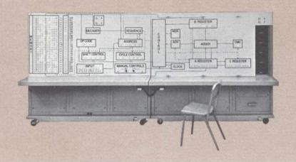
The entire twelve foot face of the system is used to display in flow diagram form the operation of a small-scale general purpose computer.
