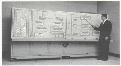
When operating as a computer trainer, the entire 12-foot unit is used to demonstrate in block diagram form the organization and operation of a small-scale, general purpose computer.
