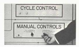
The manual control on the right enables the instructor to insert data into any particular memory location or to load the entire memory in sequential address order. The left control enables the instructor to select one of four run modes. A switch is also provided to enable the instructor to execute the program from a remote location.
