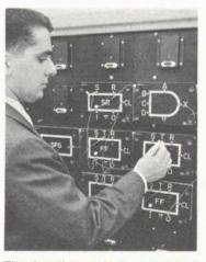
The function and characteristics of every block or subassembly on the flow diagram panels can be easily explained by actually building these subassemblies with the appropriate logic modules.
