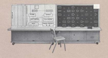
The trainer converts quickly to a detailed logic demonstrator. The removal of three of the Computer Trainer's display panels exposes a mounting panel which can accommodate up to 53 independent logic demonstrator modules.
